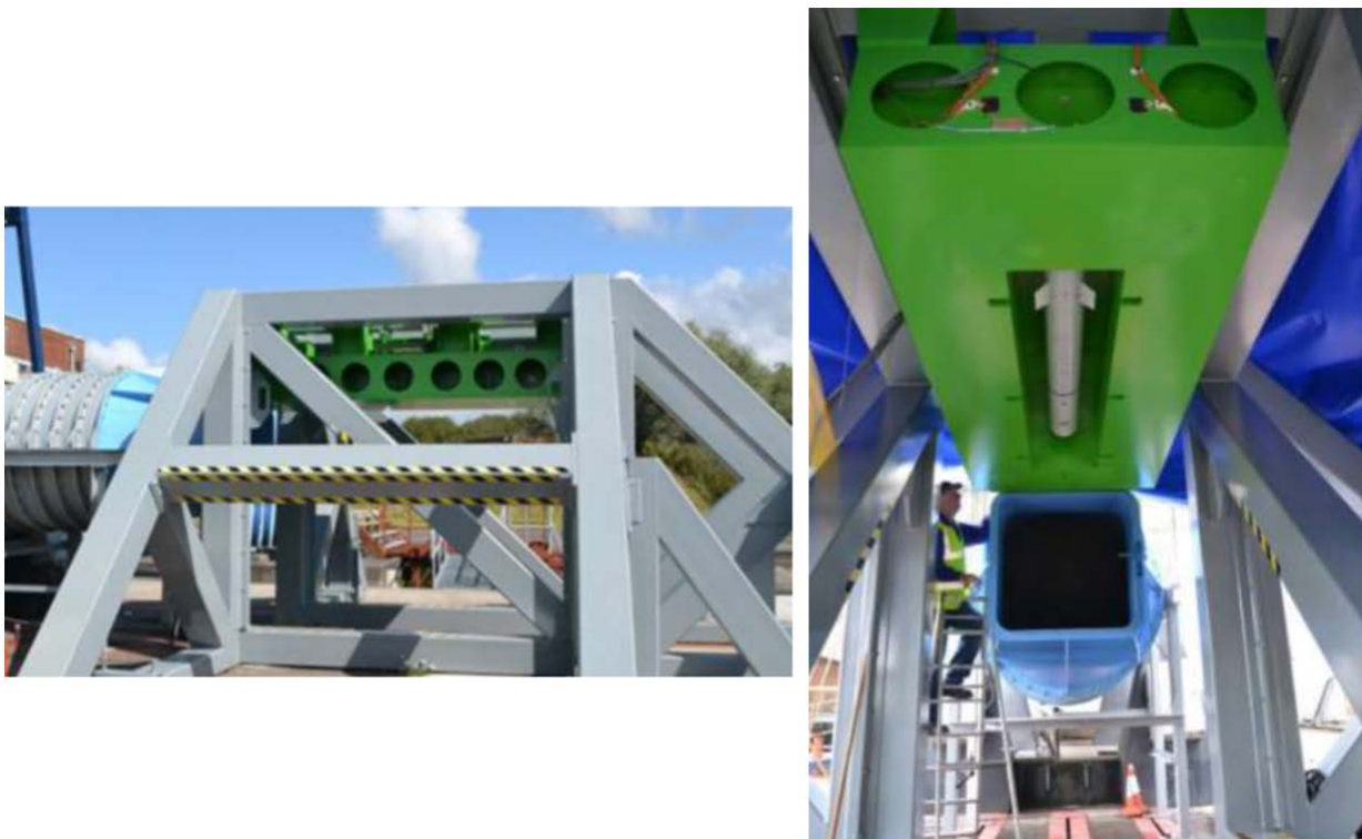
Figure 23-4: (Wind-off) Photographs of the weapon bay rig installation at the High Speed Blower Facility at BAE SYSTEMS, Warton (from [8]).
